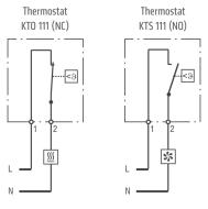
Filter fan, Cooling equipment, Signal device
